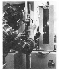
**READING THERMOMETERS** with a telescope, Irwin C. Filsinger (2411-2) calibrates the thermometers inside the vertical chamber. Accuracy achieved is within .02 of a degree.
